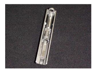
Taking the guide rod assembly in one hand, apply a small quantity of oil to the inner guide rod and smaller spring.
