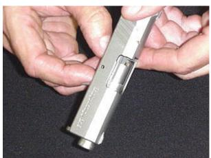
Here is the barrel fully inserted in to the slide.
