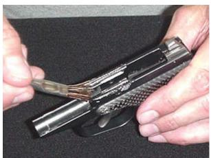
Also a grease film on the "floor" of the frame where again, the barrel chamber will be located
