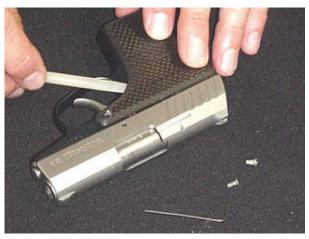
Using the aforementioned nylon tool, we see here the relief that is machined out of the right grip panel.
