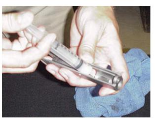
Again using the syringe of grease, we apply two small deposits onto the slide rails, one each side. Here seen just forward of the ejection port and close to Eric's index finger tip.
