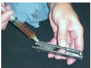
Once that oil has been applied, it can be usefully distributed as a modest film with the index finger as shown here.
