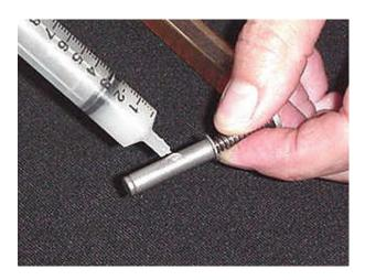
Using again the brush approach, distribute the grease over the entire surface of the main guide rod.
