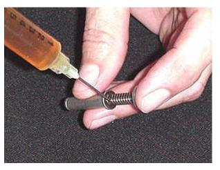
Place a small drop of oil on the main guide rod.
