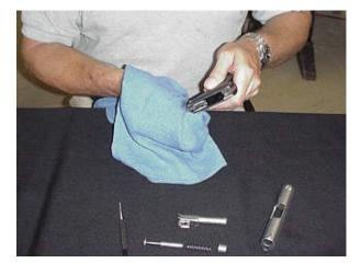
The barrel next - and this must be cleaned of course externally, including the barrel lug slot.
