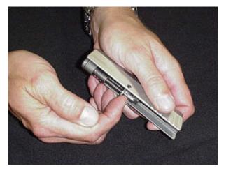
Once the rear disk is clear of the barrel lug then slowly allow the spring tension to release - taking care to avoid any parts flying into distant corners of your room!.
