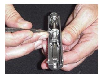
The disk position has now been lowered slightly - bringing it parallel to slide long axis - and it can also be seen that left and right positioning is good.
