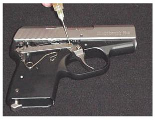
Lastly we can apply another small amount of oil, to the coiled area of the trigger return spring.
