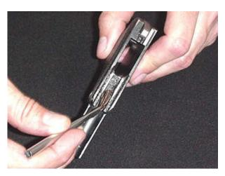
Finally, with the frame, the rails need to be lubricated - fairly generously. The brush makes distribution of the grease a lot easier and helps avoid local areas of excess.
