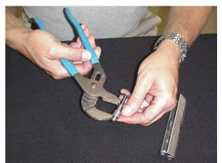
With the recoil assembly secure in the pliers, offer up the end of the main recoil guide rod to go through the hole in the slide end.
