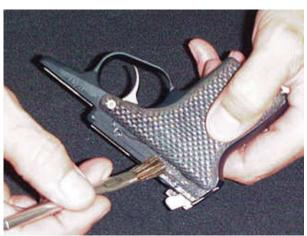
Just another view of brush-distributing grease, over the rails on the frame.
