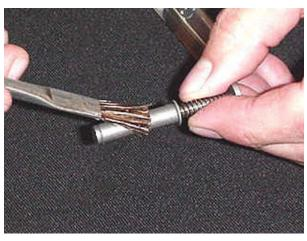
Time now to replace the large recoil spring over the main guide rod.
