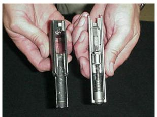
The next stage is to remove the recoil assembly and for this the hold shown in the photograph is probably the best.
