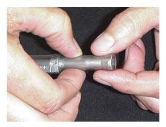
We can now replace the barrel into the slide.
