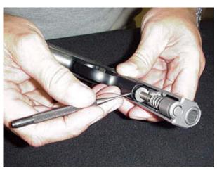
To check adjustment and location of the rear disk on the barrel lug - view the assembly as shown here, and a look from the side can be useful too.
