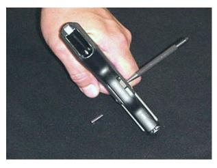
With the punch removed, it is an easy matter to withdraw the slide forwards on the frame thus separating the two parts.
