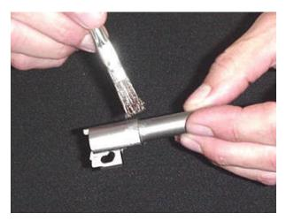
Moving on - we need to apply grease to the barrel lug slot. This is most important as it rides over the pin during operation.
