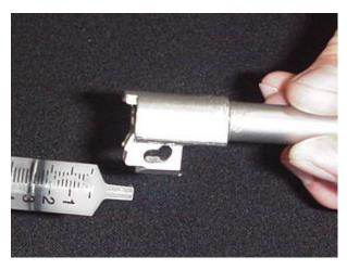
Using the brush again, we distribute the grease evenly over entire surface of the barrel lug slot, and even over the lug itself.
