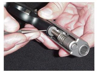
This is where (punch pointing) the rear disk of the recoil assembly impinges on the frame.
