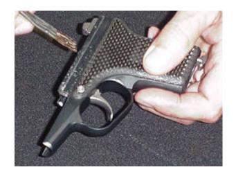
To replace the complete recoil assembly is best achieved by use of Channel Lock pliers.
